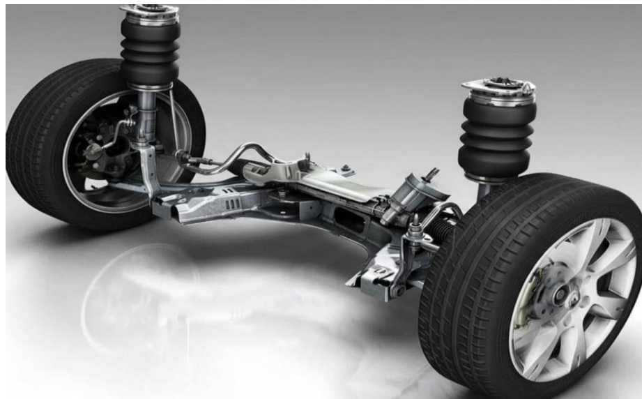
Figure 8: The state of a spring shock absorber after it has been converted into a bellows-type shock absorber.
