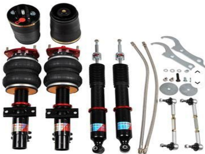
Figure 5: Air bellows, shock absorbers, hoses and fittings.
