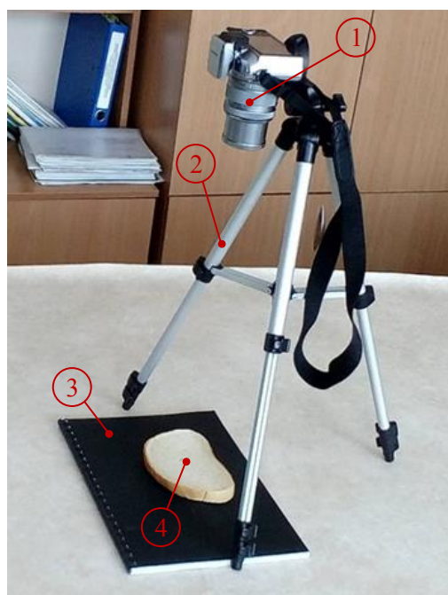
Figure 1. Experimental setting for the images capturing: 1- digital camera; 2 – a tripod for holding the camera in a stable position; 3 – black pad for background unification; 4 – a bread slice.
