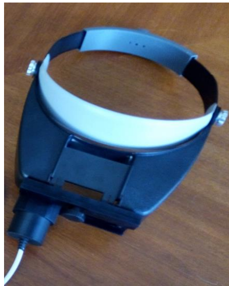
Figure 2. Photo of the prototype of the apparatus - component that allows functional attachment of the UV light source to the head of the patient.
