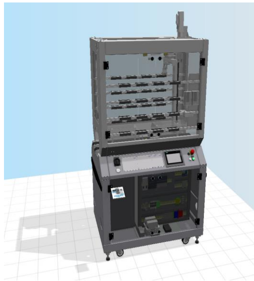
FIGURE 2. One module of the CP Factory is our testbed which is described and studied in this contribution (store of pellets with 2D manipulator) the ASRS32 module.
