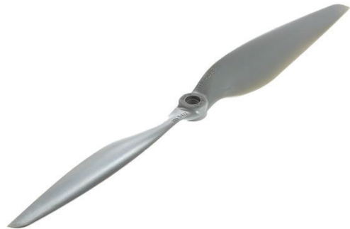
Fig. 5. Propeller APC 10x4.5
