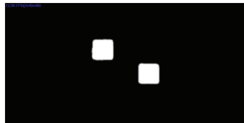
Fig. 4. Output After Threshold Filter
