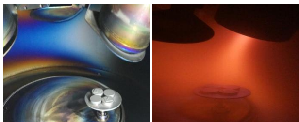
Fig. 1. The substrate holder location and plasma in vacuum chamber during deposition process.
