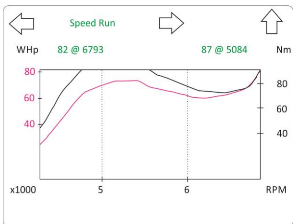
Fig. 11. Power and torque of the spark ignition engine operating with LPG and switched off advance processor.
