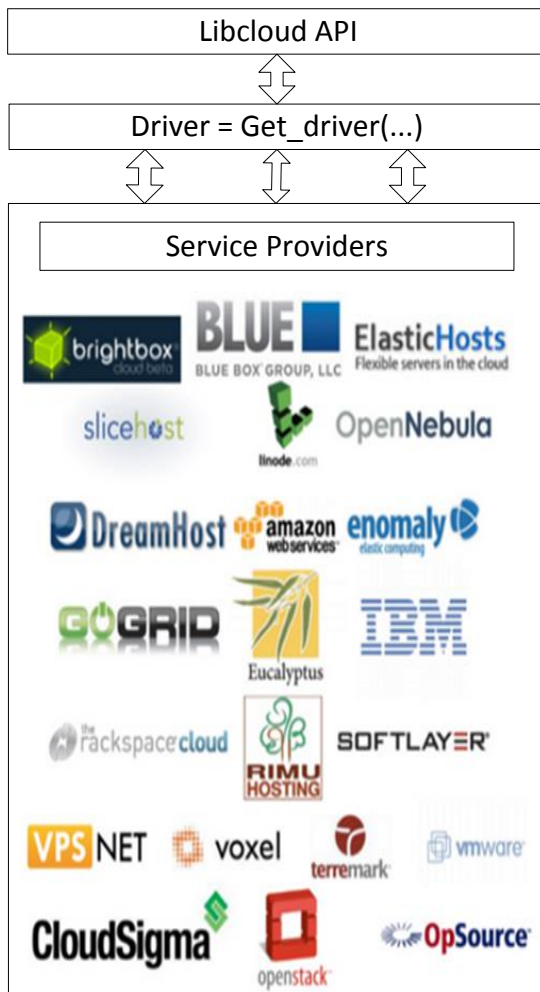
Fig. 1. Accessing different cloud providers through Libcloud API
