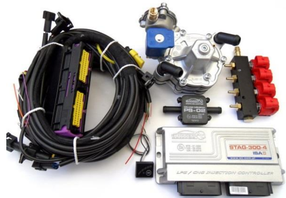
Fig. 1. Front kit of LPG system
