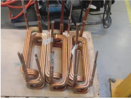
Fig. 9. MKC coils after impregnation
