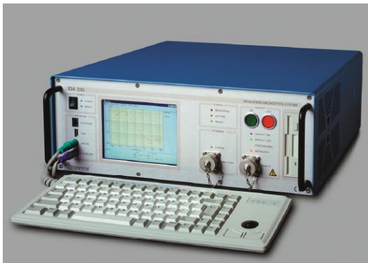
Fig. 2. Insulation diagnosis system equipment
