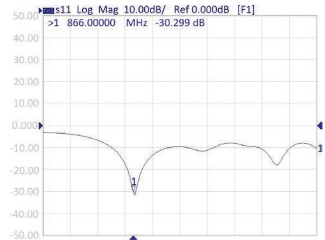
Fig. 11. The Impedance matching of the dipole antenna over EBG structure
