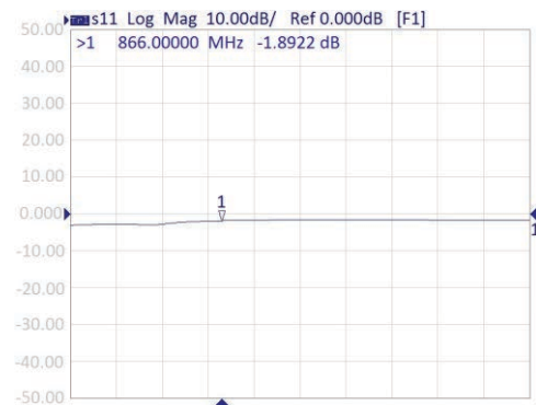
Fig. 8. The Return loss of the dipole antenna over ground plain sheet metal reflector
